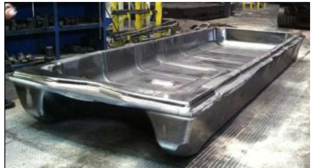
Figure 1. Joint-less demonstrator component produced from forging process for US Army RDECOM (now DEVCOM) ManTech Program.
