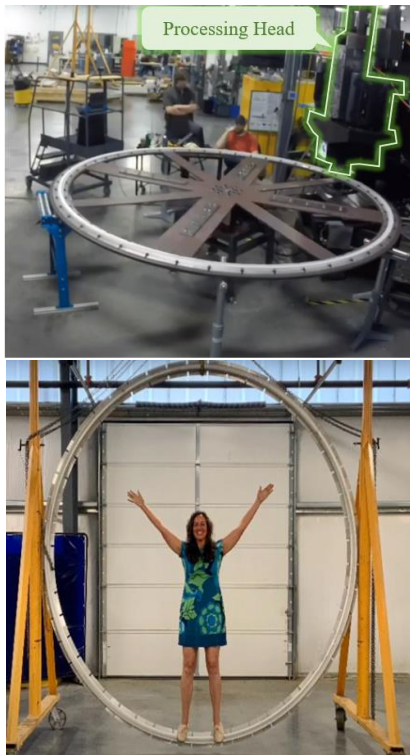
Figure 4. Example of large scale component printing (top) and end result (bottom) [8].
